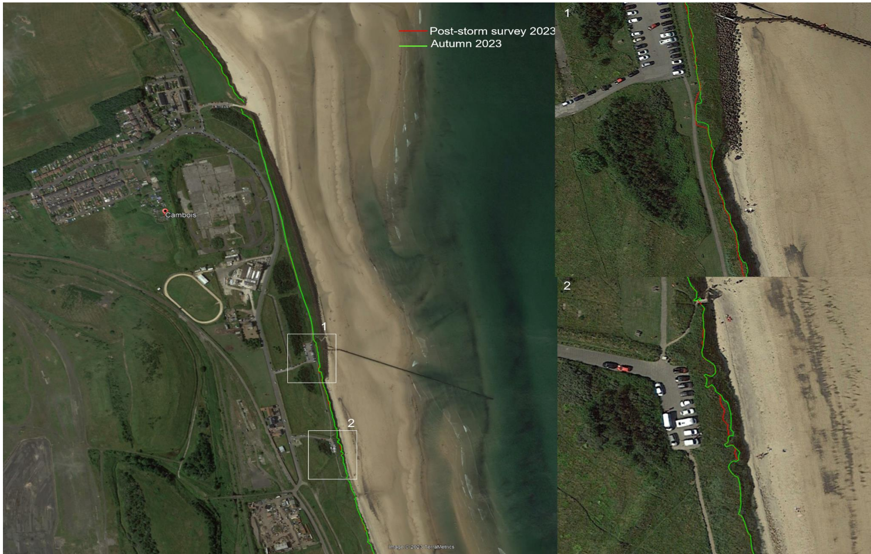
Figure 3 Cambois Bay cliff top surveys in Autumn 2023 (pre-storm survey) and November 2023 (post-storm survey) – North of bay
