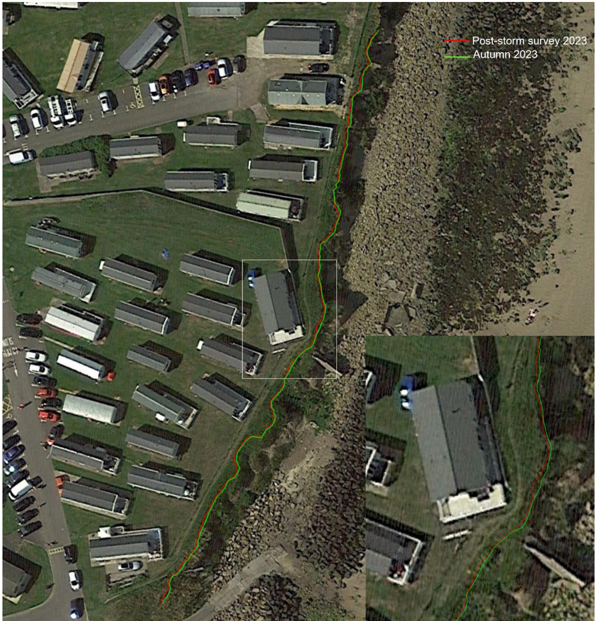
Figure 2 Cambois Bay (Sandy Park) cliff top surveys in Autumn 2023 (pre-storm survey) and November 2023 (post-storm survey)
